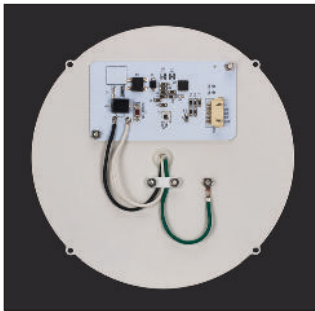
On-board IC drive technology – no external driver needed
